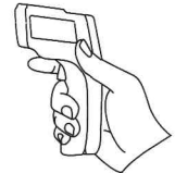
RELEASE to lock the temperature result
