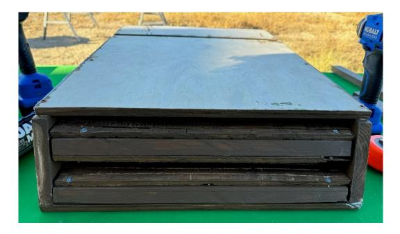
Caulk around all top surfaces, sanding first if necessary to ensure a good fit with the roof. Attach roof to sides and roof supports with 1 1/4" screws, and finish by caulking around the roof and side joints to protect the bats from any wind or rain that might get into the box.
