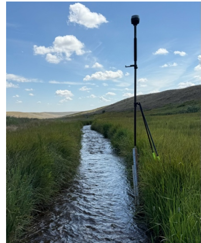
MTSRN being used to measure the location of a staff gage for Greenfields project.
